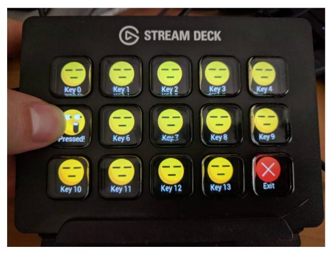
This is an open source Python 3 library to control an Elgato Stream Deck directly, without the official software. This can allow you to create your own custom front-ends, such as a custom control front-end for home automation software.
